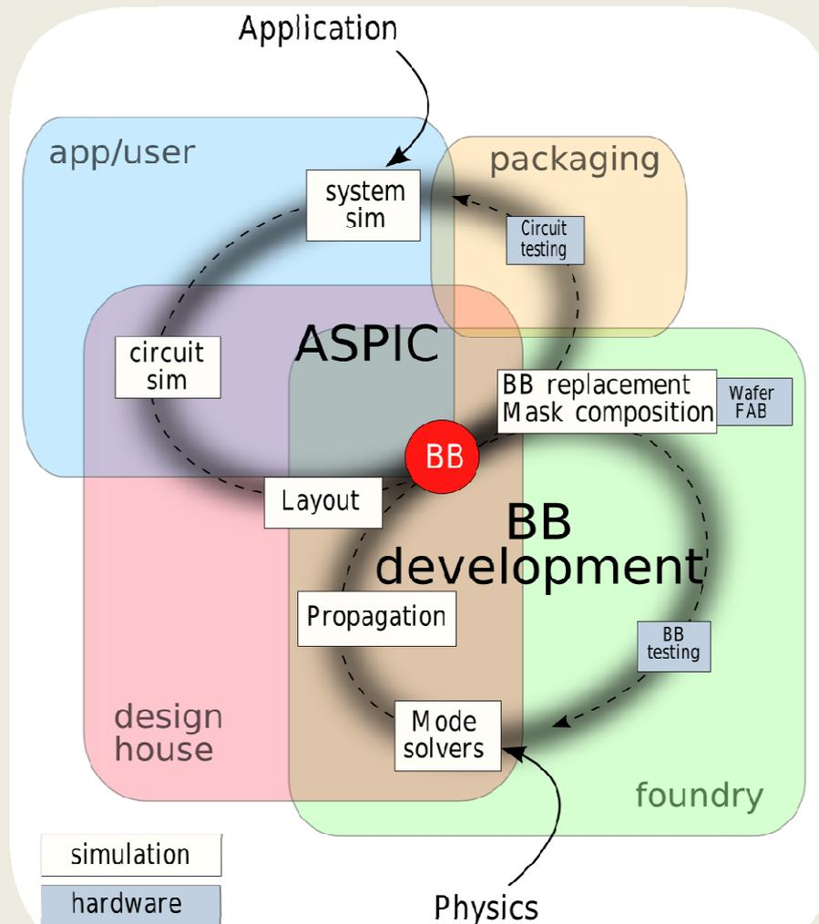
Figure 1 Two main design flows in the generic InP process, the "ASPIC" loop and the "BB development" loop. BB denotes a photonic Building Block. The rectangles identify the four main stakeholder groups.
